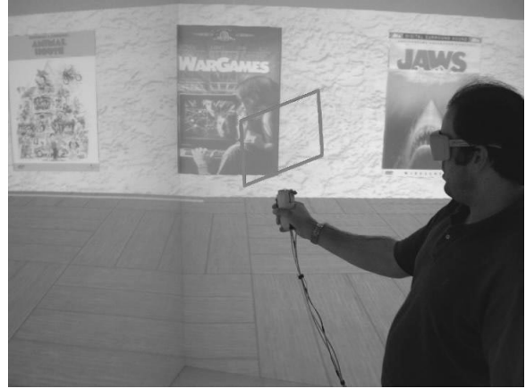
Figure 4. With the SnapShot technique, users invoke this cropping widget with a light pressure on the trigger button. A firm pressure takes the snapshot of the area seen through the widget frame.
