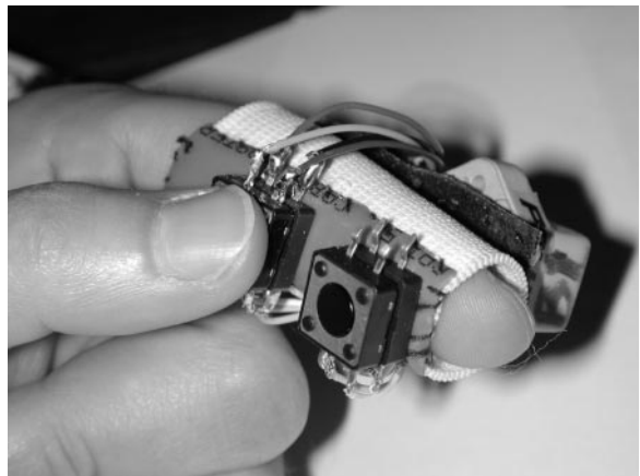
Figure 1. The FingerSleeve device mounts two small pop through buttons on an elastic frame, with the tracker placed on the back of the sleeve.
