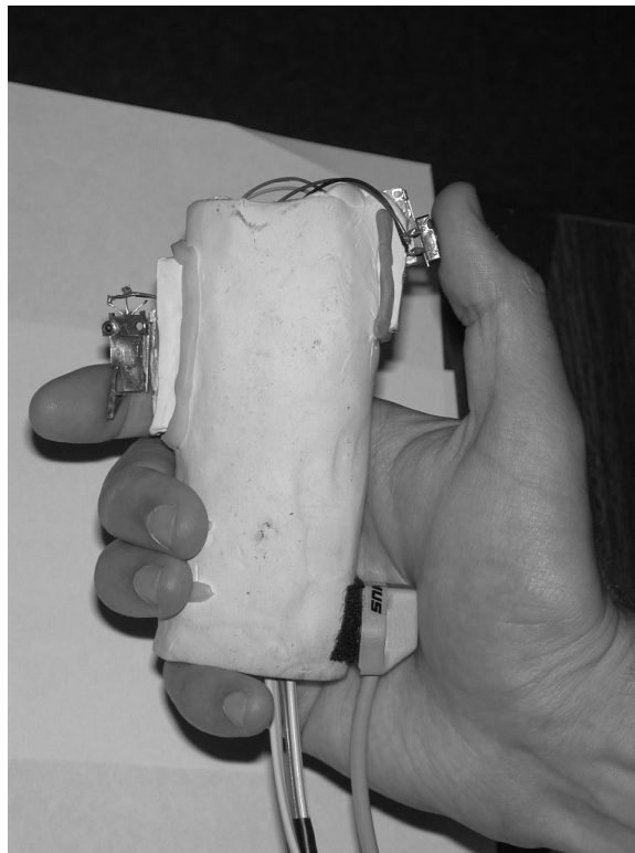
Figure 2. The TriggerGun device houses two pop through buttons mounted on a modeling clay frame. One is placed on the front to be used as a trigger, and the other is placed on top for thumb activation.
