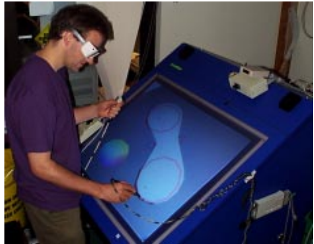
Figure 1: A user creates 3D geometry at the ActiveDesk with a pen and performs camera operations using the 3D tracker in his non-dominant hand.
