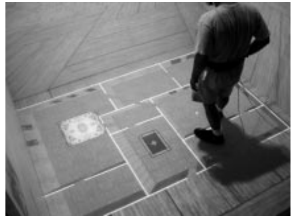
Figure 2 The Step WIM widget which allows users to quickly navigate anywhere in the virtual world. The small sphere by the user's foot indicates his position in the miniature.
