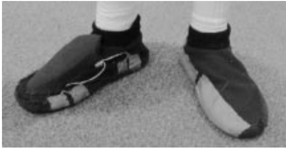
Figure 3 The Interaction Slippers allow the user to tap either their toes or heels to trigger Step WIM functionality.
