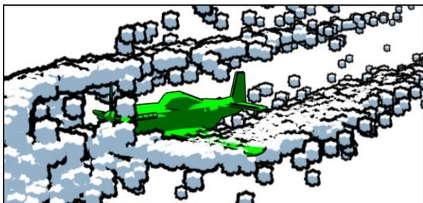
**Figure 3.** Clouds deflected by collisions with an airplane and swirling from interaction with propeller blades and vortices.
